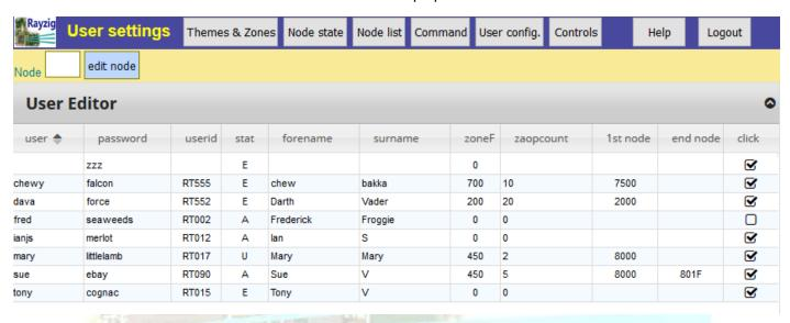
The details are set up such that the Restricted user is assigned a primary zone (Zone F) and also a block of output modules. Once these are defined, access can be given to the user, and they can control these. So, User Sue, is able to control up to 32 modules with Module Addresses of 8000 to 801F, that are assigned to Zone 450. Sue is able to define 5 Themes and 4 Zones.
